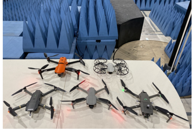
Figure 5: All UAVs that we used in our study. From top left, i) Autel EVO II, ii) DJI Mavic Mini, iii) DJI Mavic Pro, iv) DJI Mavic Air 2, and v) DJI Mavic 2 Pro.
