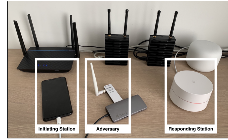
Figure 5: Experimental setup, depicting a Google Pixel 4 XL and Google Wi-Fi AP as an initiating and responding station.
